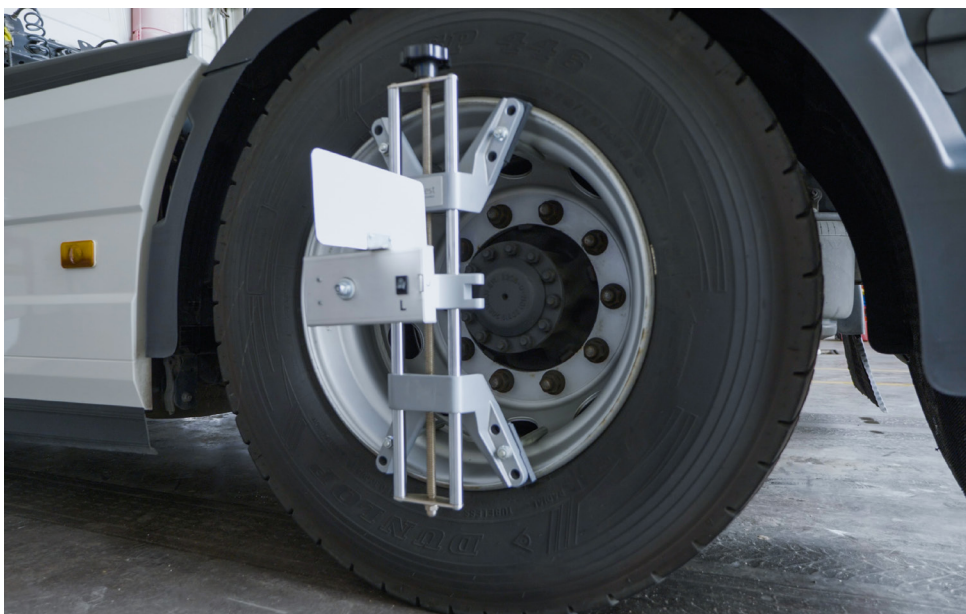
Wheel centering connection tools
