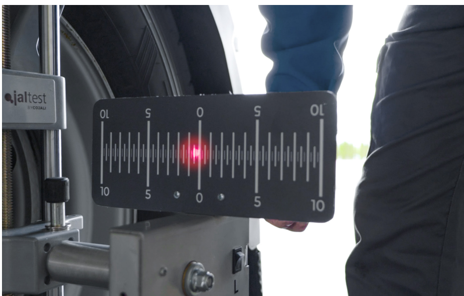
Measuring scales of the wheels
