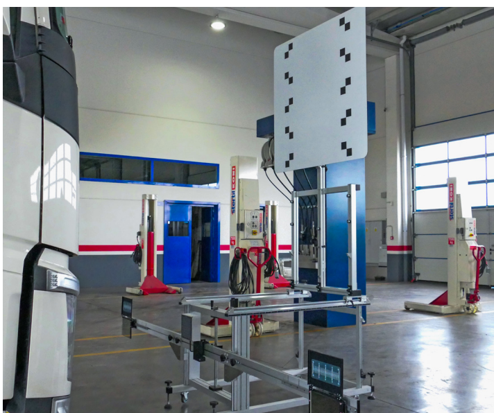
General image for information purposes with the calibration target for Volvo FH V4
