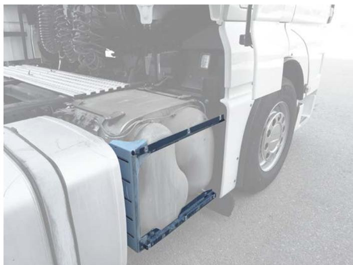
**d.** Disassemble the AdBlue/DEF injector fixing and remove the injector.
