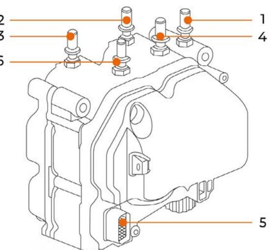
**c.** Connect hose “**7**” with quick coupling of 3/8” to the AdBlue/DEF intake connector **(6)**.
