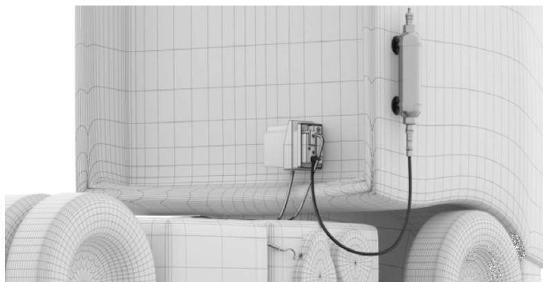
**f.** Fill tank “**2a**” with 250ml of hot distilled water (MAX. 60°C/140°F) from the upper part.
