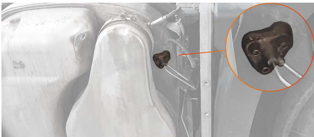
**d.** Place a container under the injector nozzle.
