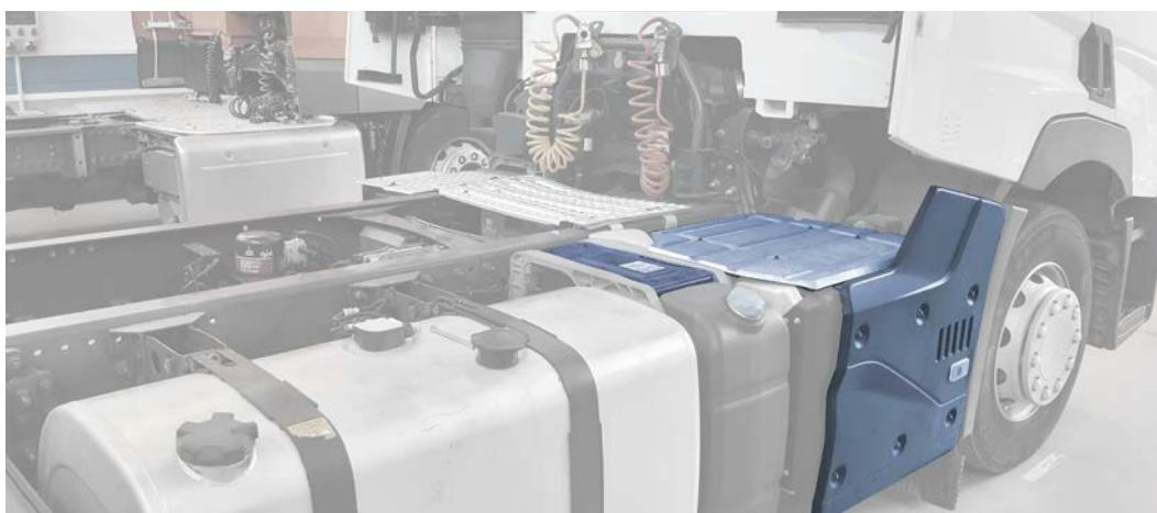
For greater comfort during the process, disassemble also the support of the side plate.
