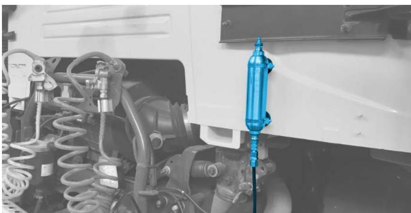
**f.** Fill tank **“2b”** with hot distilled water (60°C/140°F MAX.) from the upper part, using the filling bottle **“6”**.
