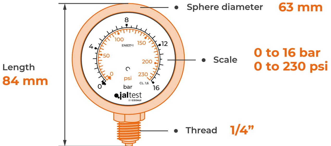
Pressure gauge suitable for pneumatic installations. The glycerin dampens pressure peaks, mechanical impacts and vibrations, apart from protecting the mechanical components of the pressure gauge and enabling precise reading.
