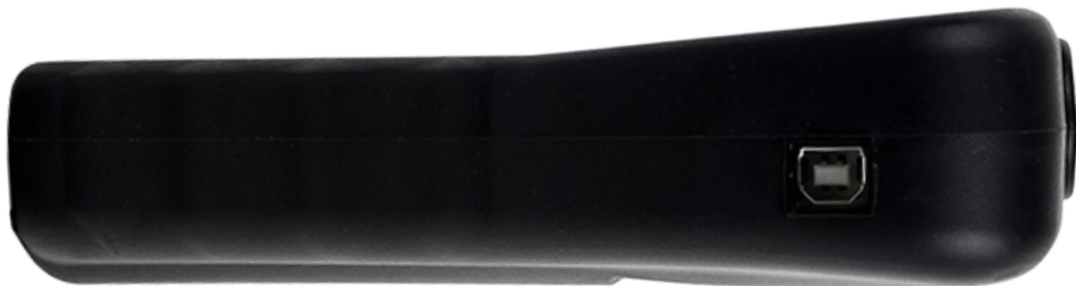
USB connector for battery charge and software update.
